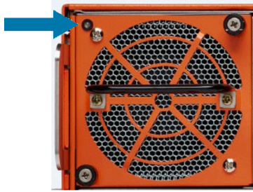
Figure 6 Individual Fan LED Location on GigaVUE-HC3 Rear
