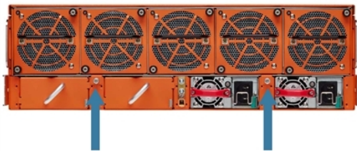
Figure 10 Fan Tray Screw Location on GigaVUE-HC3 Rear
